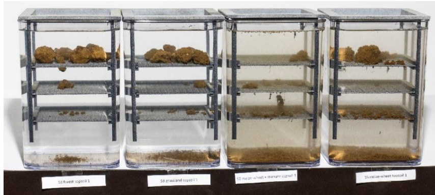
Slake test: wet macroaggregate stability in site B. Sieves with 10-, 5- and 2-mm size with soil aggregates of 15-20 mm in size immersed in water. Stable aggregates remain on top sieve (first two), while unstable aggregates disintegrate (third and partially fourth)
